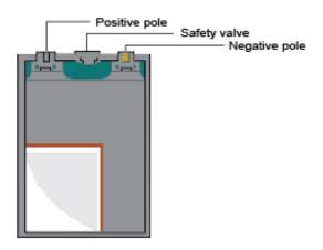
Drawing2 Lithium-ion power battery structure drawing
