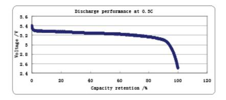
Drawing3 Lithium-ion power battery discharge curve
