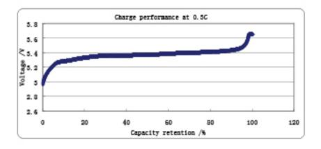
Drawing3 Lithium-ion power battery charge curve
