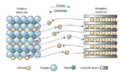
Drawing1 Lithium-ion power battery charge/discharge schematic diagram
